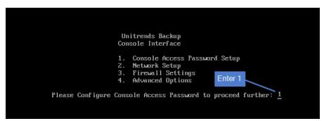
3 To change the direct console password, enter a new password, then enter the password again to confirm.
