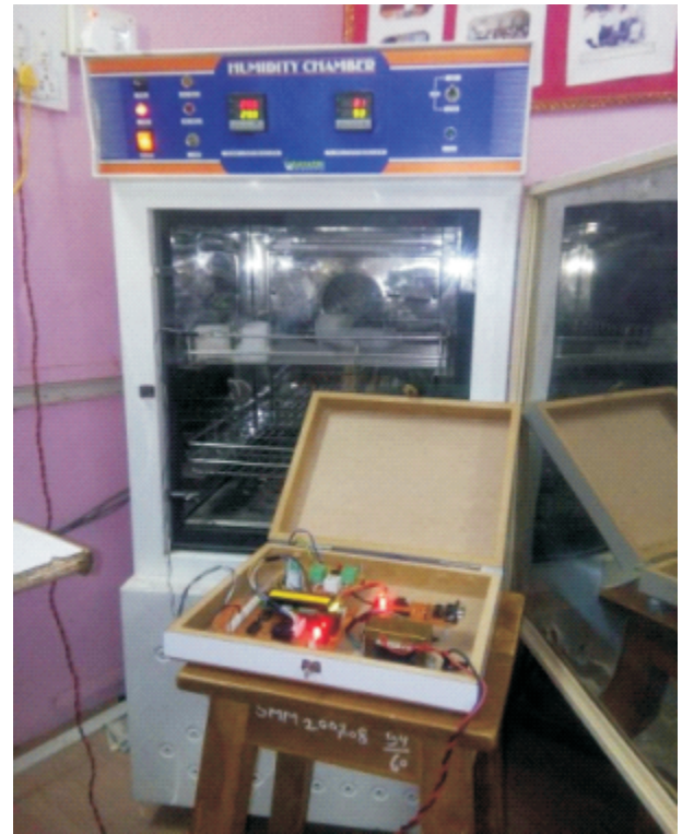
Figure 11. Experimental Setup Calibration of System for Humidity
