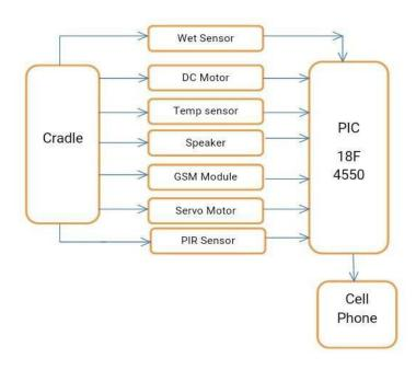
**Working-** When child is ready for sleep in cradle various sensor like noise sensor, PIR, wet sensor ,temperature sensor are used to monitor the child .firstly if the baby is in cradle the system is activated. When baby is crying the noise sensor gets input and system activate the music through Speaker and swing cradle is performed. Swing of cradle is performed by servo motor and toy start rotating due to DC motor.
