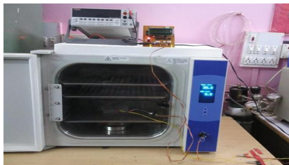
Figure 4: Experimental arrangement for calibration of the sensor module for CO 2 in %.
