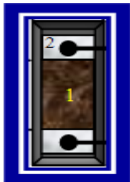
Figure 2: The schematic of the sensor fabricated by using ferrite material under investigation
