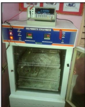
Figure 3: Experimental arrangement for humidity dependent resistance measurement.
