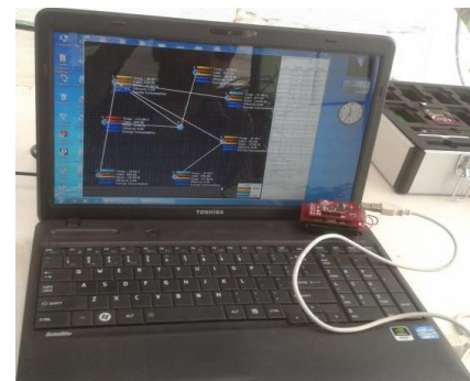
Fig.25. Photograph showing establishment of Base Station of WSN-HBEX
