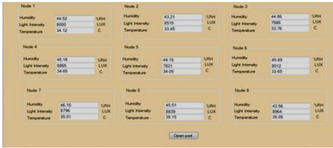
Fig.13. The Photograph of GUI developed in VB environment to demonstrate the Site-Specific Data Collaboratively collected by the WSNodes of the WSN designed for Polyhouse
