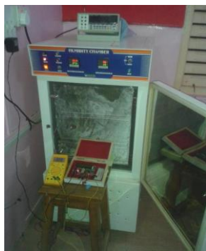
Fig.14. Experimental arrangement for calibration of WSNode for Humidity in RH%
