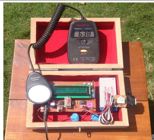
Fig.18. Experimental arrangement for calibration of WSNodes for Intensity of Sun Light in LUX using standard LUX meter Mastech make MS6610
