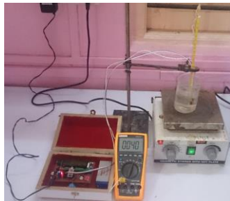
Fig.16. Experimental arrangement for calibration of the WSNode for temperature in °C
