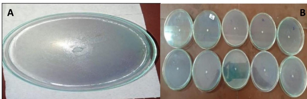
Figure 3 Test of antibacterial activity using disc diffusion assay (quantity per disc -10 μ) A) for R8D, B) for all synthesized 5-aryl-[1,2,4]triazolidine-3-thiones.
